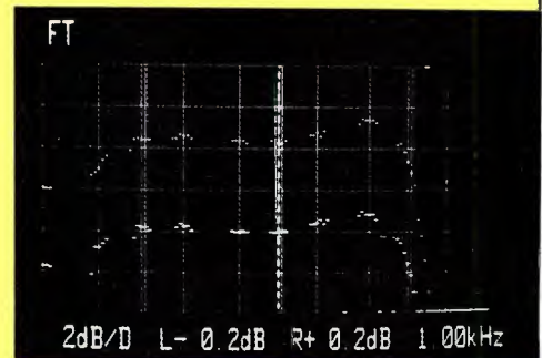
Figure 2. A CRT display of spot frequency measurements using the instrument. The system can generate a fast, segmented frequency response sweep from 40kHz to 20Hz. Placing the cursor bar at a point on the CRT trace will generate the alphanumeric data of frequency and level.
