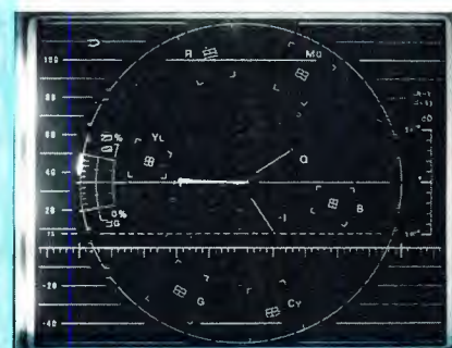
Figure 8. A timing jitter of about 6ns peak-to-peak on the selected signal's sync on the SCH display.
