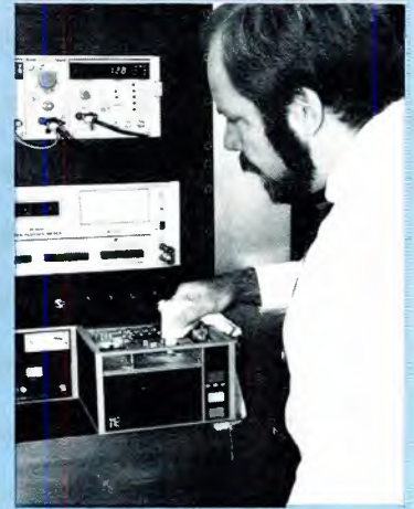
The author demonstrates the correct procedure for cleaning a ceramic capstan shaft.
